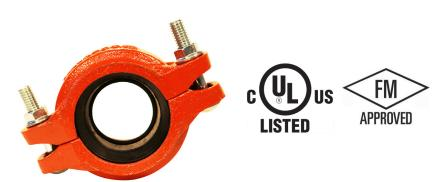
The ARGCO Model 105 reducing coupling allows for direct reduction on a piping run and eliminates the need for a concentric reducer and couplings. The specially designed rubber gasket helps prevent small pipe from telescoping into larger pipe during vertical assembly.
